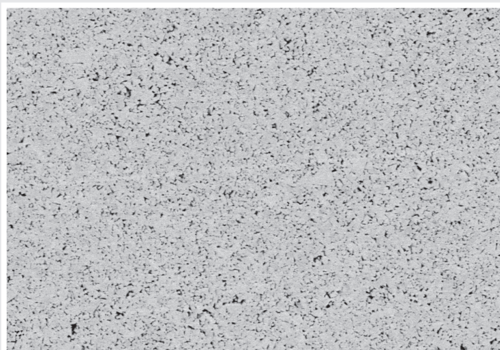
Grade HB-110 submicron grain, 90/10 (carbide / cobalt %) for general-purpose tool making.
